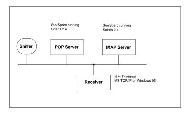
Figure 2: Experimental Setup for Delivery
