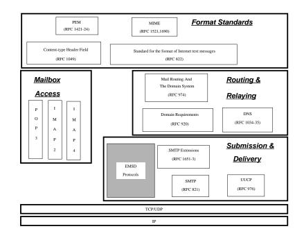
Figure 6.4: Messaging Communication Stack and EMSD
