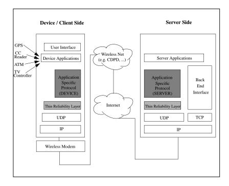
Figure 5.1: Anatomy of a Vertical Wireless Application
