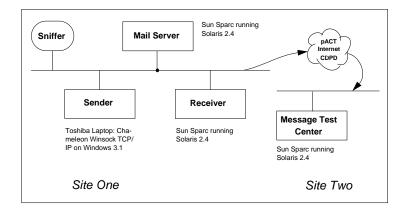
Figure 7.1: Experimental Setup for Submission
